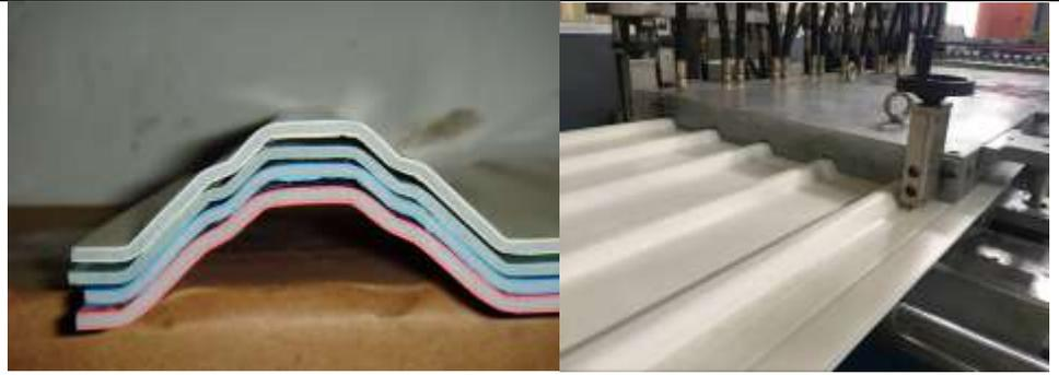
Three layered Foamed Roofing Sheets
