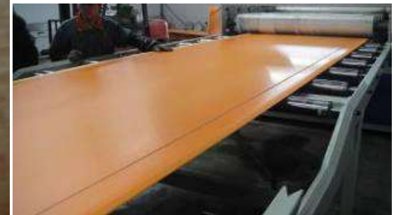
PVC Foamed board and Wood +PVC Solid Board making
